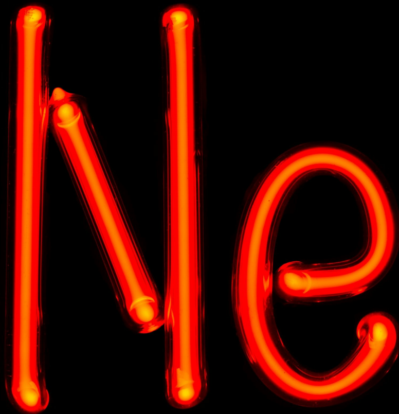
Neon gas discharge tubes (arranged to spell out the atomic symbol for Neon, Ne)
